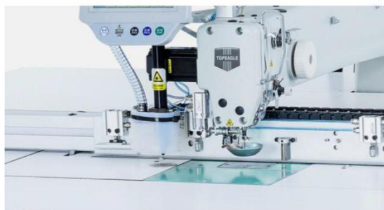
The laser function is used to pocket welting, repair the flap, and repair the collar.
